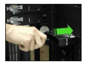
7. Push the tray lever until it clicks, and secures the drive tray in place. The drive tray is correctly placed when its front edge aligns with the bay edge.
